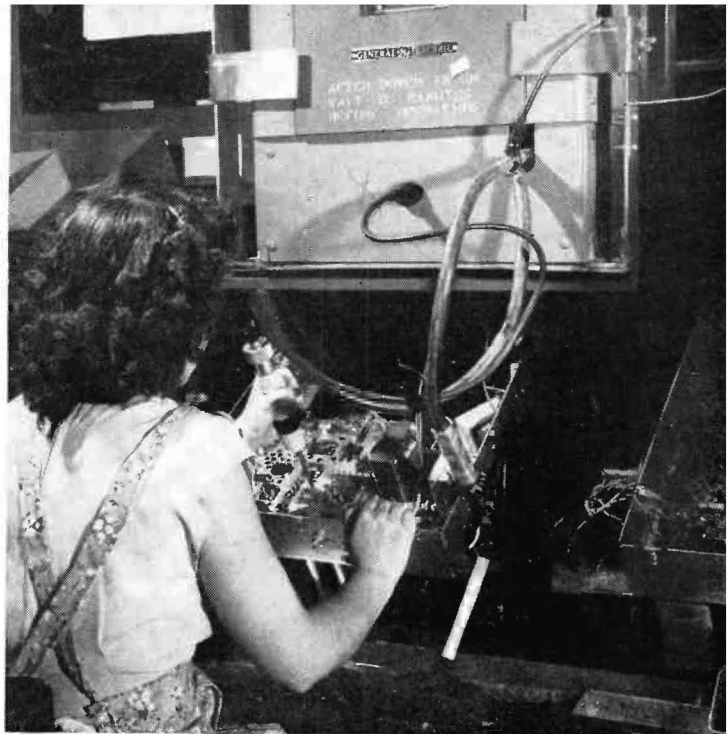
WELDING REPLACES SOLDERING —With electronically controlled resistance welding, this operator is able to weld 15 grounding ribbons and one resistor lead to the chassis of a television set during the two-minute time cycle. A snap-action switch built into the welding electrode applies current automatically
