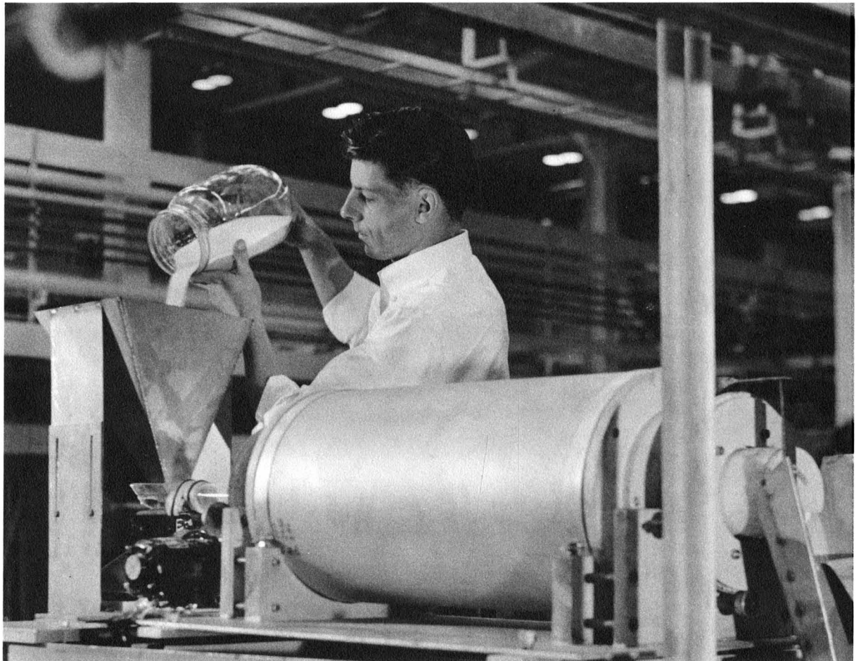
Ceramic powder is poured into a continuous-mixing, rotating-muffle furnace for purification.
