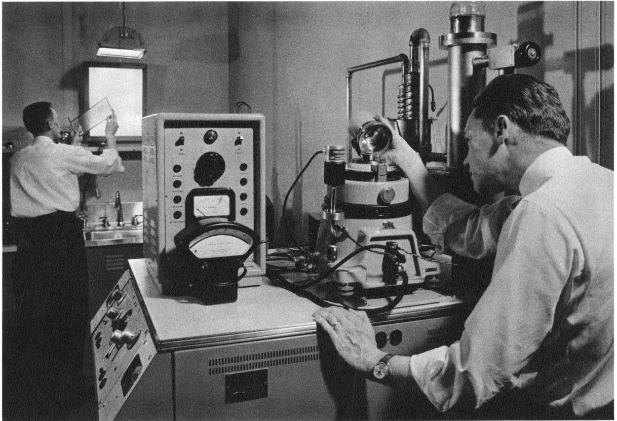
Crystal structure of alloys can be studied by means of a special high-temperature x-ray camera.
