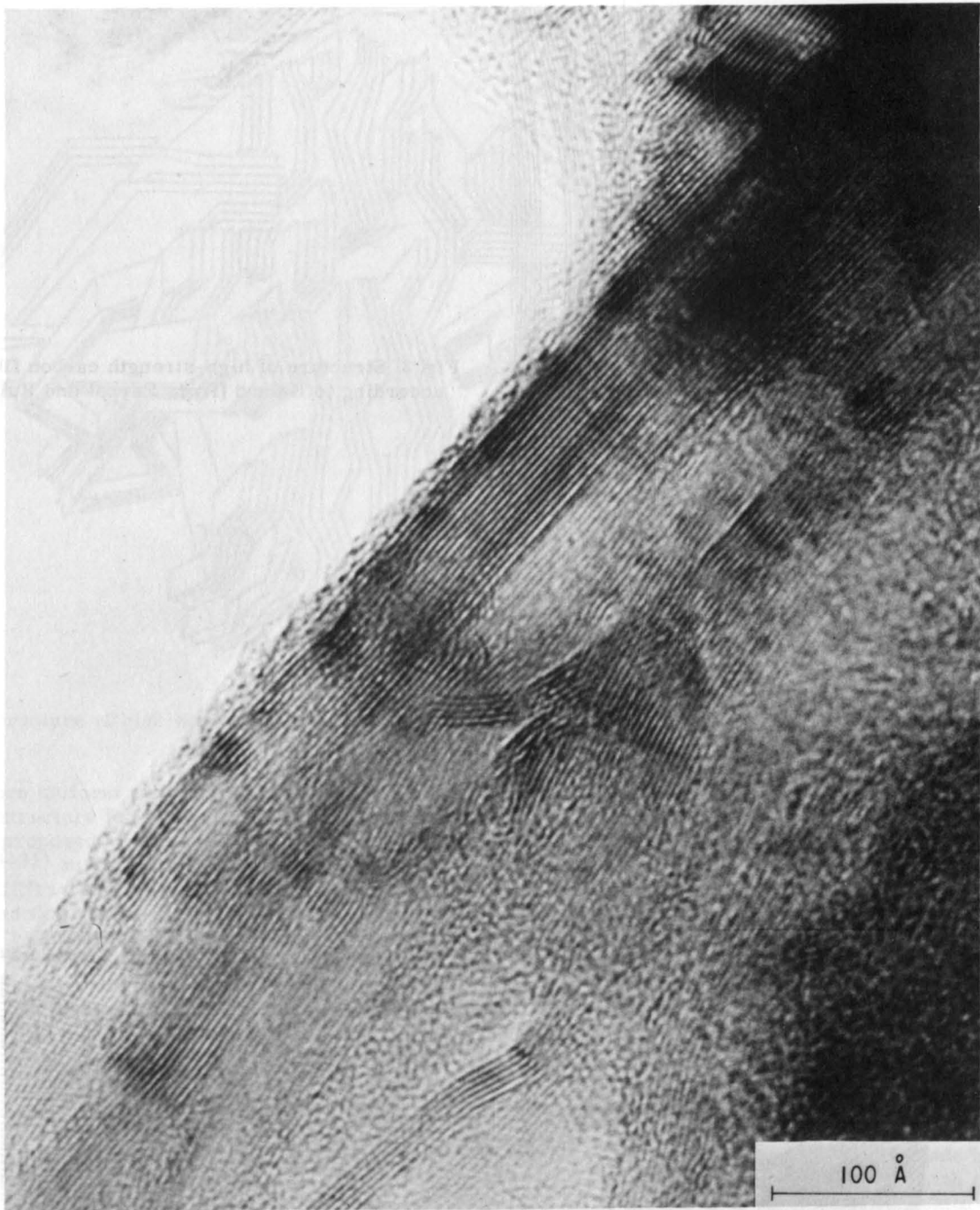
Fig. 5 Transmission micrograph of PAN-based Type I carbon fiber. (Courtesy of V. A. Phillips, General Electric Company.)
