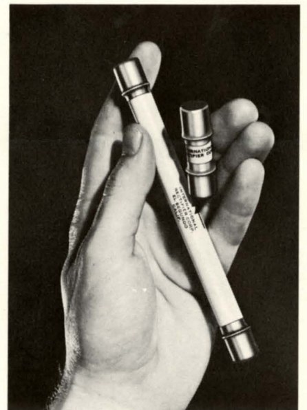
International Rectifier was the first to design and develop this configuration for ceramic encased silicon cartridges. Rated to 16,000 volts PRV — up to 440 ma @ 75°C, they feature ferrule ends for insertion into standard fuse clips. Request Bulletin SR 225 for ratings on 36 standard types.
