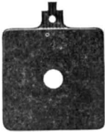
Fig. 1 A single Kuprox disc—a complete rectifying unit in itself. This piece of solid copper Kuprox metal permits an electric current to pass through it in but one direction.
