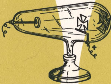
modified Crookes Tubes... forerunner of the modern cathode-ray tube
