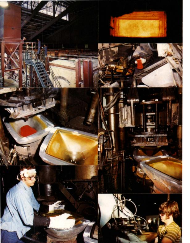
The mixture formulated for either the panel or the funnel is delivered to its furnace 9 where the mixtures are melted 10. For the funnel-making process, a portion of molten glass 11 is drawn from the furnace, cut off, and dropped into the funnel mold 12. A shaping plunger enters the mold and is then withdrawn 13. After blasts of cool air are applied, the hot funnel is removed from the mold 14 and the neck is formed 15.
