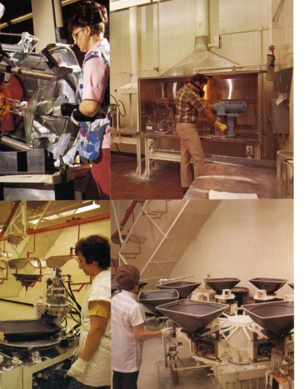
After inspection, a coating is applied to the inside of the neck 22. The frit material, which is mixed 23 in small batches, is applied to the lip of the funnel 24. Then, after another washing 25 the funnel is ready for attachment of the panel.
