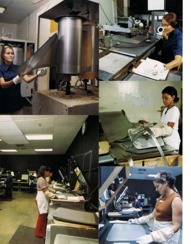
One mask is then stripped from the roll 19 and inspected for aperture size at several locations 20 across the mask. The finished masks are individually stripped from the roll 21 and each one is inspected 22 23 for aperture position, size, and shape.
