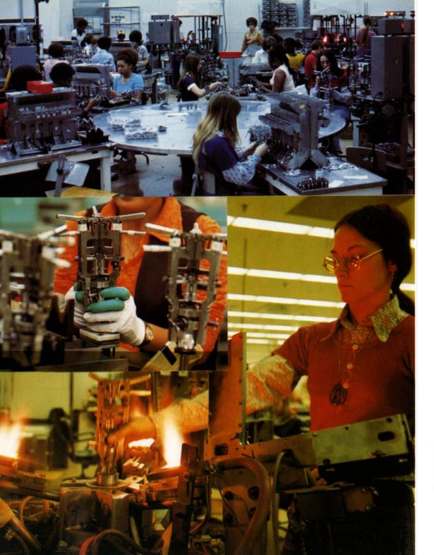
These various parts are assembled with a special fixture around a revolving work table 17, and when completed 18 each assembly is bonded by beading with flame 19.
