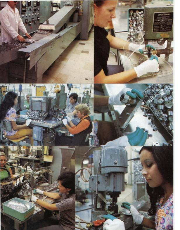
They are further decontaminated by firing in a hydrogen atmosphere 7. After this step great care is taken to assure against recontamination. Special gloves and finger tip coverings are used throughout the subsequent processing 8. The assembly process includes several sequential welding steps 9 10 11 12.
