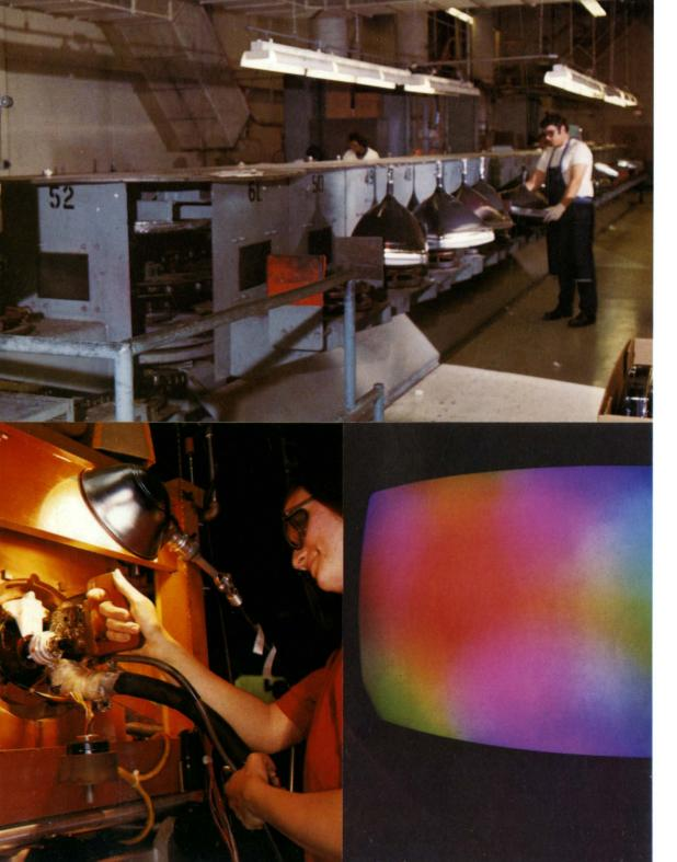
The final steps in the tube processing are varied to optimize production efficiency and to suit the needs of particular tube configurations. Here is shown the application of a conductive coating to the tube envelope 7, assembly and adjustment of the precision in-line yoke 8, and a preliminary characteristic test 9.
