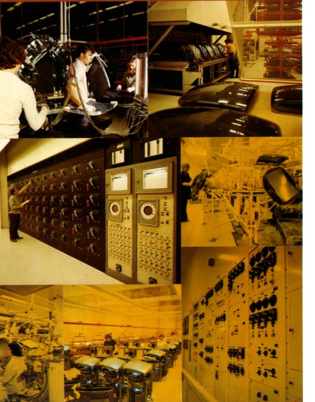
The panel is then transferred to the assembly line where the mask is accurately positioned on the panel studs 33. Then, after another trip through the stabilizing Lehr 34, controlled from a single board 35, the panel goes to the slurry room 36 where the three phosphors are applied 37 and the locations set by an exposure on the light-house stands 38. In the slurry room, the electrical controls are centrally located so that the entire operation can be monitored and checked from one position 39.
