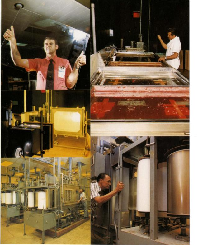
The special master 9 is maintained and duplicated in the dark room facilities 10 11. After the photographic exposure, the roll of steel is developed in a special process 12 which cleans the aperture pattern and coats the balance of the steel with an etch-resist so that only the aperture pattern is affected. Close inspection 13 assures that the processing is adequate.
