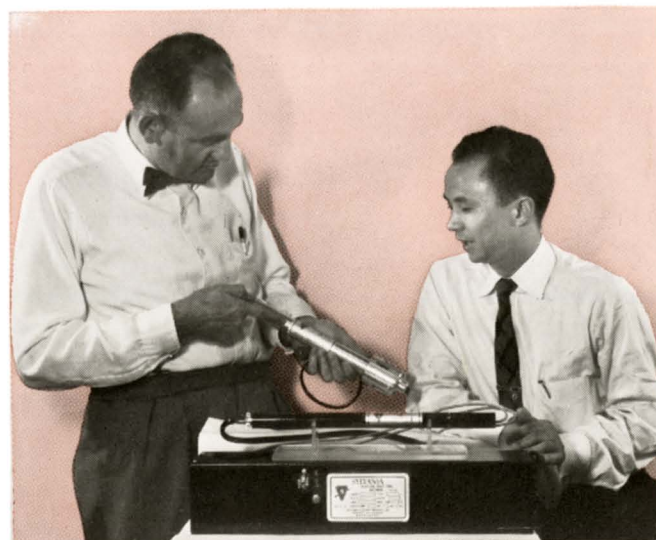
Scientists examine light-weight traveling-wave tube, new device with large military and commercial potential.
