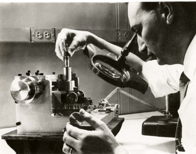
Materials of extremely high purity and special electrical characteristics are required for semiconductor devices such as transistors and diodes. (above) Pure silicon being produced for research. (below) Measuring characteristics of silicon and other semiconductor materials.
