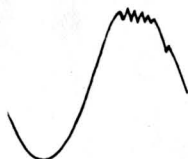
Fig. 25.—Output wave-form showing "buzz" effect.
