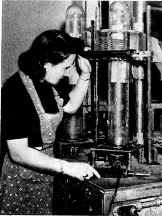
Fig. 5—Induction-heated vacuum firing station.
