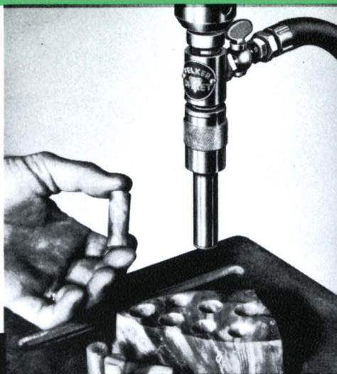
PETRIFIED WOOD and other semi-precious stones are easily cored for inspection and interior coloration. Cores can be sectioned, ground and polished for settings.
