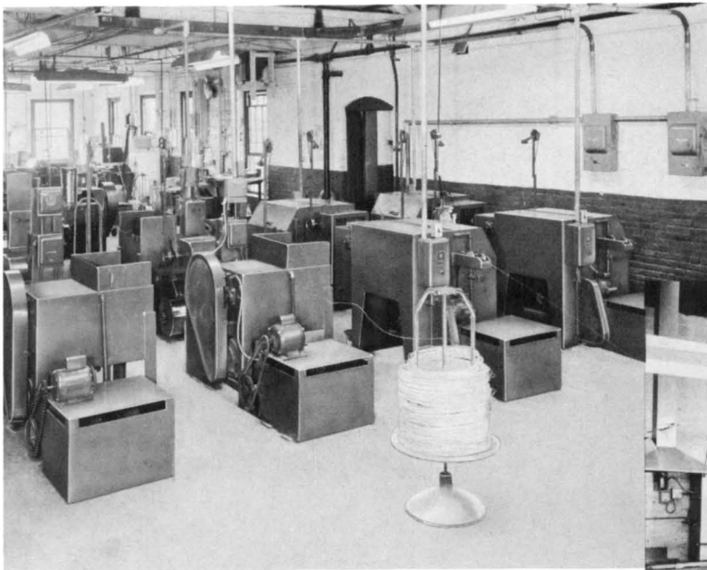
Intermediate wire drawing units with a diameter range from .057" to .011".
