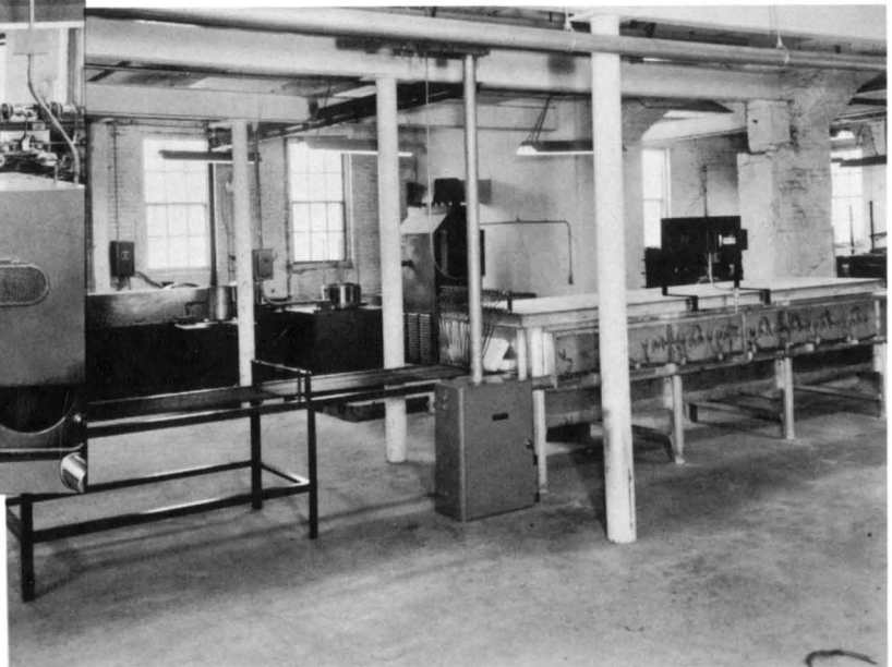
Additional heavy wire annealing furnace with diameter range from .125" to .050".
