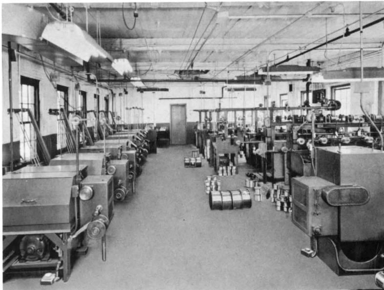
Fine wire drawing section of plant with a diameter range of .040" to .001".
