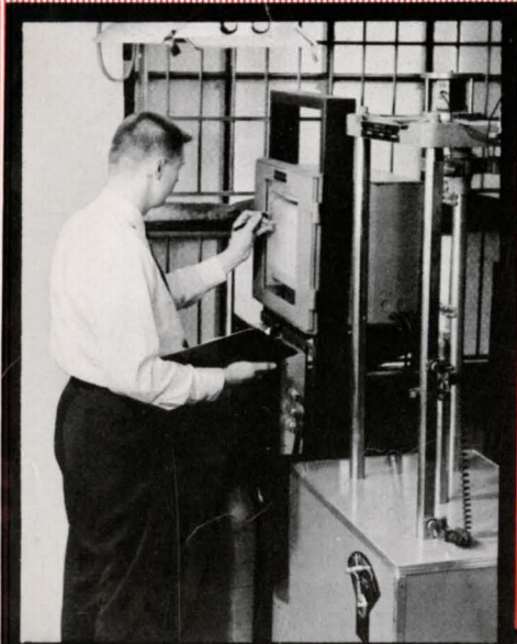
Constant rate of strain tensile tester in a section of our physical testing laboratory.
