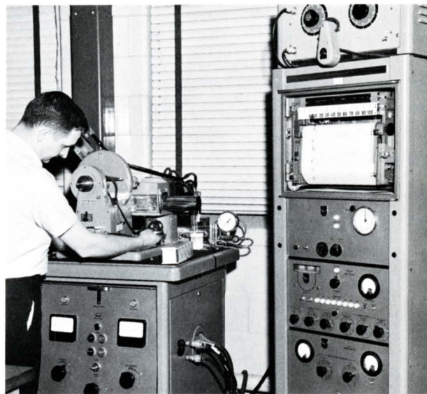
X-ray diffraction unit, set up for measuring thickness of nickel plate on molybdenum wire.
